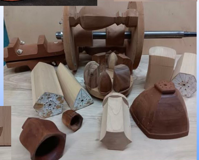
Brian frequently experimented with ways to get non-round shapes off the lathe. This pursuit led to the development of a therming jig, his "lost and found" wood technique, and square bowls.
