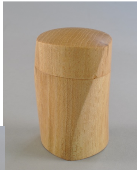
three-sided, Twisted, Lidded box, turned on 4 axes: One axis for each side, and hollowed on the original axis.
