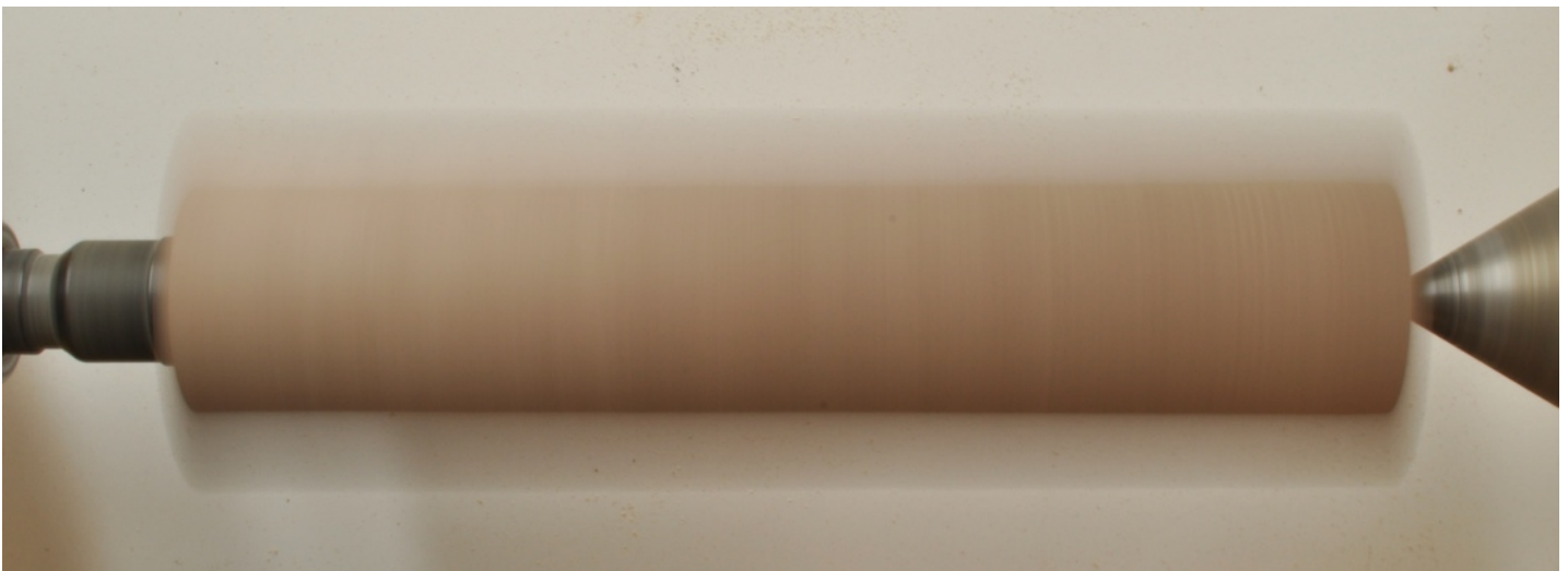
The bias created by an axis parallel to the original axis produces a uniform shadow across the work.
