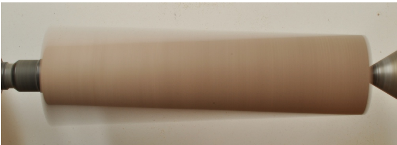
The bias created by an axis intersecting the original axis will produce a diminishing shadow along the work. The second axis on this work was effected by shifting (only) the center on the headstock (left), such that the intersection of the axes is at the end of the work (at the tailstock).
