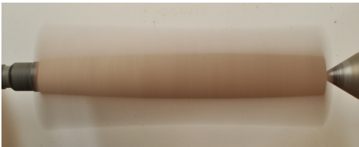
The bias of a skew axis produces a shadow that has a slight cove. Notice also that the solid wood looks like a slight bead that is a mirror image of the shadow's cove.
