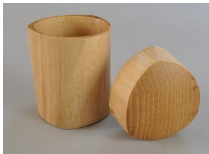
three-sided, Twisted, Lidded box, turned on 4 axes: One axis for each side, and hollowed on the original axis.
